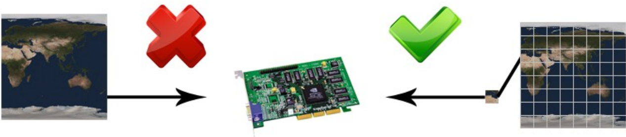
Figure 1: Partitioning the virtual texture into smaller pieces that fits in video memory.
